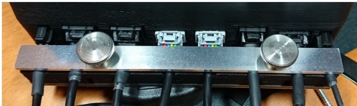
Led6 Pilot display Power Left sensor Right sensor Button box GPS Audio repeater
