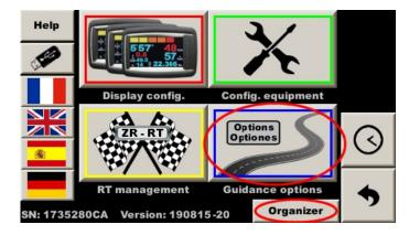
Then the GPS correction function must be enabled in the guidance options page of the main menu. If the checkbox "GPS dist. correction" is not present, the option has not been validated, please contact us.
